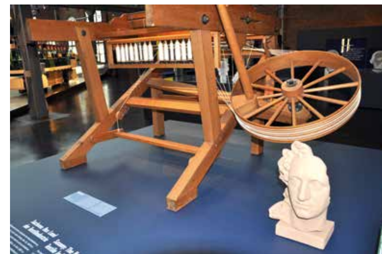
Chemnitz (Germany), Sächsisches Industriemuseum – Industriemuseum Chemnitz, replica of a historic original yarn-spinning jenny. This museum installation includes a commentary interpreting and presenting the situation in the Saxon textile production industry at the beginning of the 19th century. Permanent exhibition of the Sächsisches Industriemuseum – Industriemuseum Chemnitz. The exhibition is located in a former industrial building (the Herman und Alfred Escher AG foundry) which has been adapted for museum use. Photograph Ondřej Merta, 2015.
