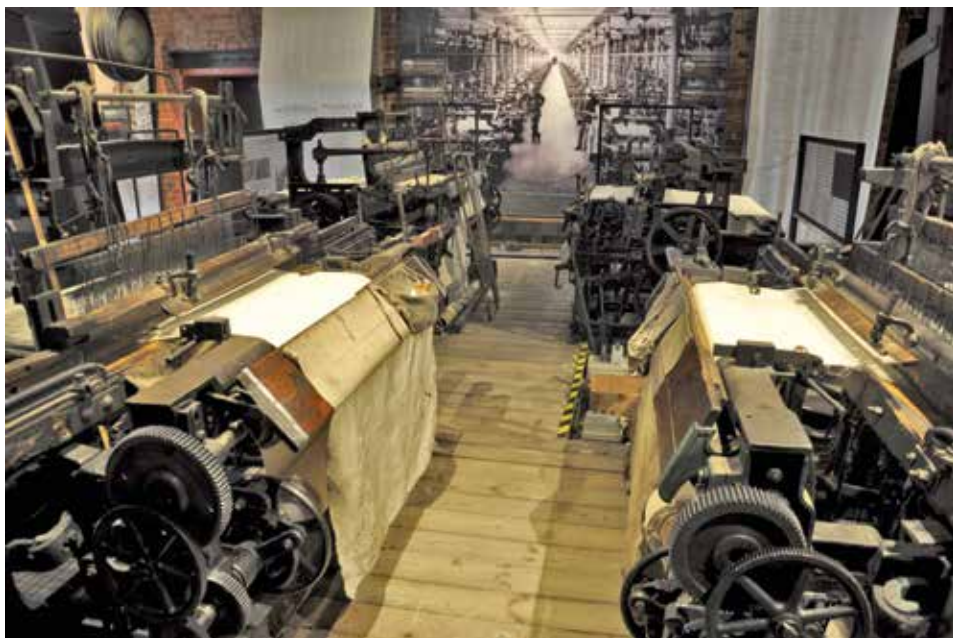
Łódź (Poland), Muzeum fabryki. An example of a new use for an industrial site where production has ceased. This museum installation at a former textile factory respects the original purpose of the building. Production machines (weaving looms) are arranged to create an exhibition interpreting the historical situation and working environment with the use of informative and illustrative materials. Photograph Jiří Merta, 2013.
