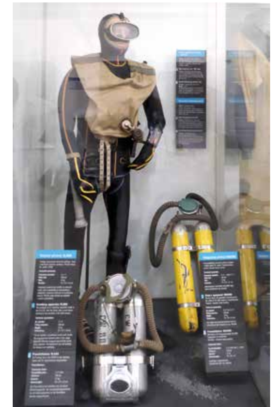
Ostrava, Lanek Park Mining Museum (Lanek Park), Museum exhibition of mine rescue equipment. Representatives of unique breathing apparatus from the diving equipment used by mine rescue workers. Photograph Ondřej Merta, 2018.
